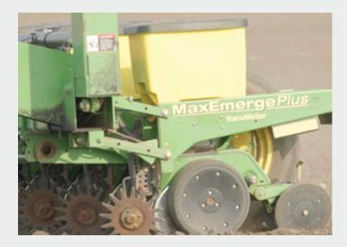
If your planter's a 3-point mounted planter you're going to want to adjust the lift arms to get the quick hitch leveled before hooking up the planter. If you have draft control on your tractor, you're going to want to turn that down or off before planting to make sure it's not trying to adjust that height and the levelness of the planter when you're going through the field.
