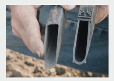
Get a tape measure and measure your guards. You want your guards to be at least <sup>3</sup>/<sub>4</sub> of an inch wide at the start of a new season. If it's less than that it's time to replace that seed tube guard with a new one, which is 15/16 inches wide. You should always replace the seed tube guards when you're putting a new set of opener disks on the planter.
