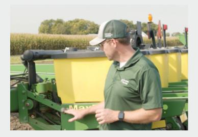
The parallel arm linkage makes sure that the row-unit is riding smoothly through the field. If there's wear in these components, you'll see that you have inconsistent depth which will lead to inconsistent emergence. It will affect spacing due to chatter in the row-unit as the planter travels through the field.
