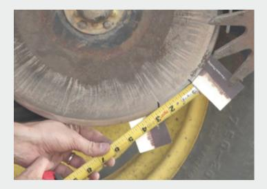
Disk openers create the furrow that seeds are placed in. To make sure that this process happens properly, you have to keep up with maintenance. Disk openers that are not maintained properly will cause erratic emergence and lost yield.
