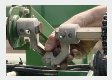
Vibration caused by mechanical components like chains and sprockets can take a properly performing meter and cause it to create skips, doubles, and spacing errors. Be sure to check the following components for wear:
