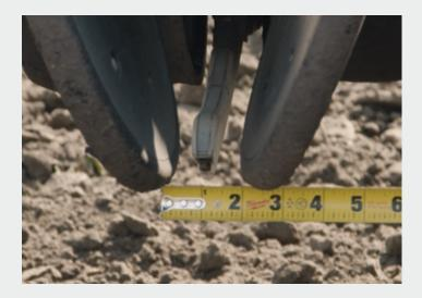
Once the seed is placed in the furrow, it is important to make sure that the furrow is closed back up with good seed to soil contact.
