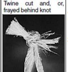
Or, Rough baling chamber slot; twine is damaged approximately 100 mm (4 inch) from knot
